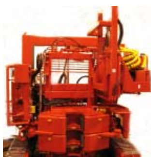
HRN 1898 front view, pipe spinner revolved
