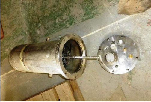
5. Emergency umbilical connection panel x 1
