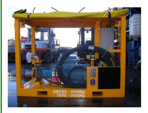
2 pole, 30Kw EExde Motor close coupled to a stainless steel centrifugal pump.
